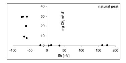
Fig. 4. Emission of  $CH_4$  as a function of Eh values in natural peat under flood conditions
