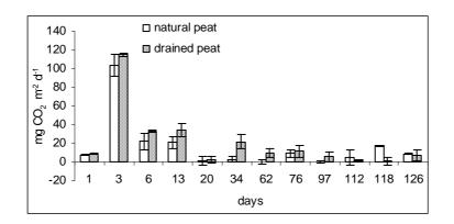
Fig. 3. The dynamics of respiration in natural and drained peats under flood conditions
