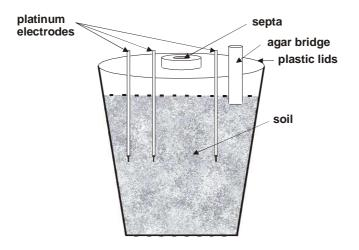
Fig. 1. Schematic of the incubation containers
